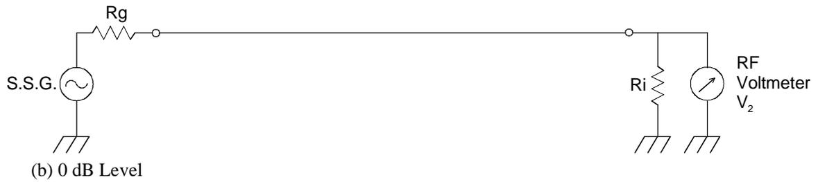
$R_g$  :  $50\Omega$  (Internal resistance of S.S.G.)
