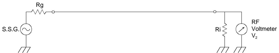
$R_g$  :  $50\Omega$  (Internal resistance of S.S.G.)
