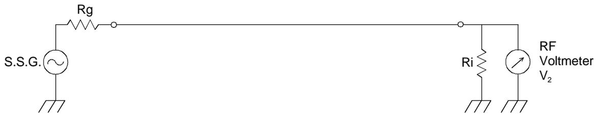
$R_g : 50 \Omega$  (Internal resistance of S.S.G.)
